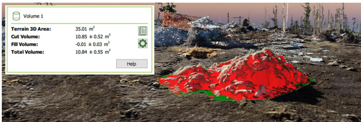
Figure 4 Volume calculation from a material pile based on drone imaging and 3D modelling (figure Juha Vihavainen).
