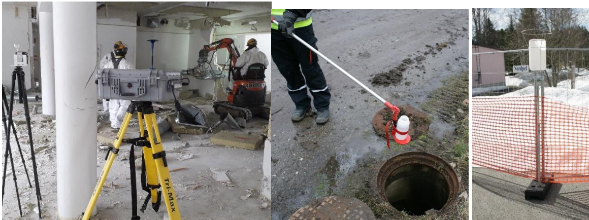
Figure 5. Real-time dust monitoring with DustTrak Aerosol Monitor during the internal demolition phase in Pankalampi demolition site (left), dust deposition collectors (middle) and water sampling (right) in Pankalampi demolition site (photos Juha Vihavainen).
