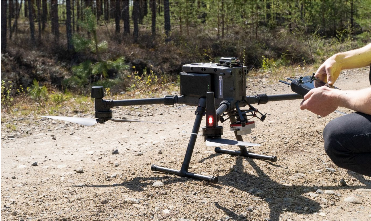
Figure 11. DJI Matrice 300 RTK drone with Micasense RedEdge-MX multispectral camera.
