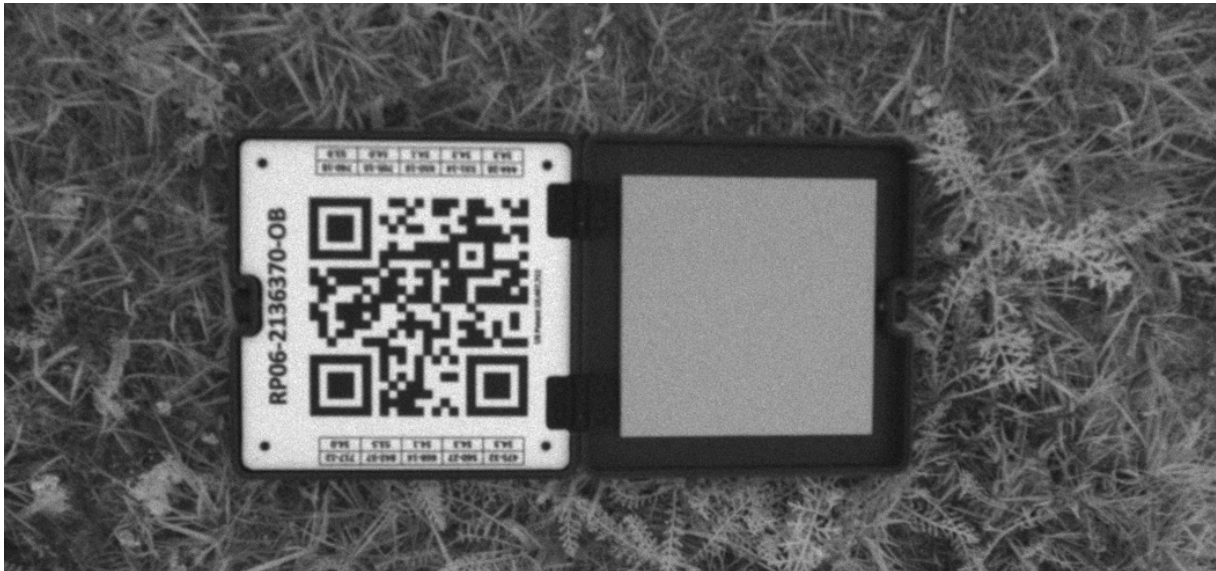
Figure 12. Picture of a calibration reflectance panel, taken with RedEdge-MX multispectral camera.
